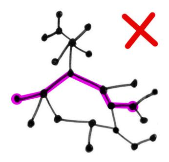
Equivalently, a tree is a **connected graph** with **no loops**.
