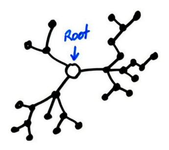
There's nothing special about the root except that it is labeled as such. Any node of a tree could be chosen to be its root node.
