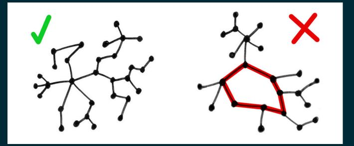
Equivalently, a tree is a connected graph that becomes disconnected if any edge is removed.
