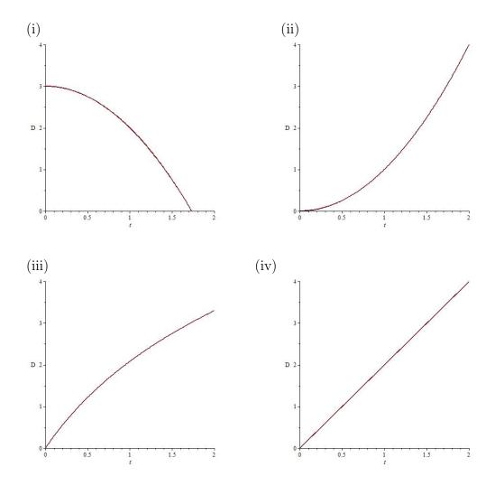
SOLUTION: (a) The graph in (iii) represents an object that is slowing down because as t increases, the absolute value of the slopes of the tangent lines are decreasing.(b) The graph in (iv) represents an object that is traveling at a constant speed because as t increases, the slopes of the tangent lines are all the same.
